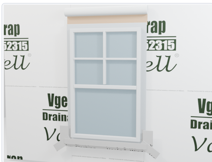
FIG 7 Set, level, fasten, and keep the sill open.
