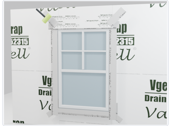
FIG 11 Tape and roll both upper corners.
