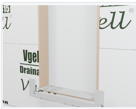
FIG 3 Install the first exterior-apron layer.
