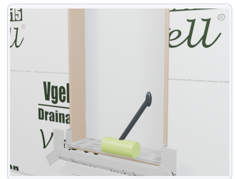
FIG 5 Add and roll the full-depth sill pan.
