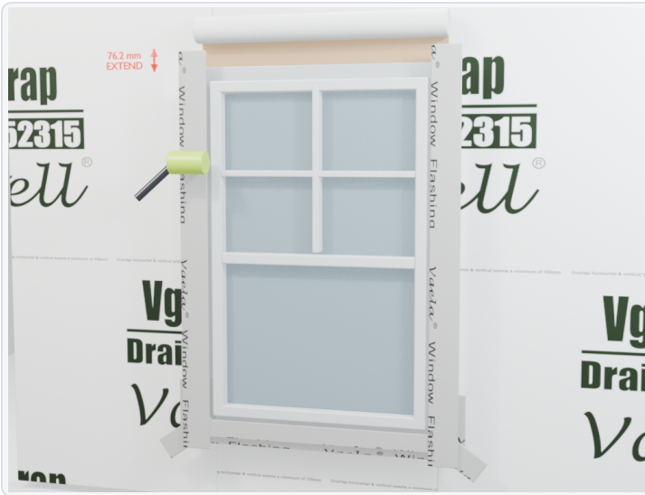
FIG 8 Apply 100 mm VWFXW over both jamb flanges.
