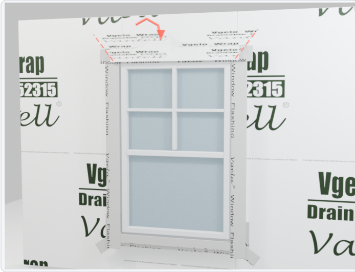
FIG 10 Fold the WRB head flap down.
