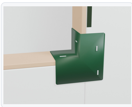
FIG 8 Install compatible preformed corner guards.
