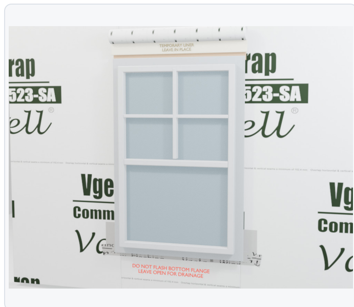
FIG 12 Set, level and fasten the window.
