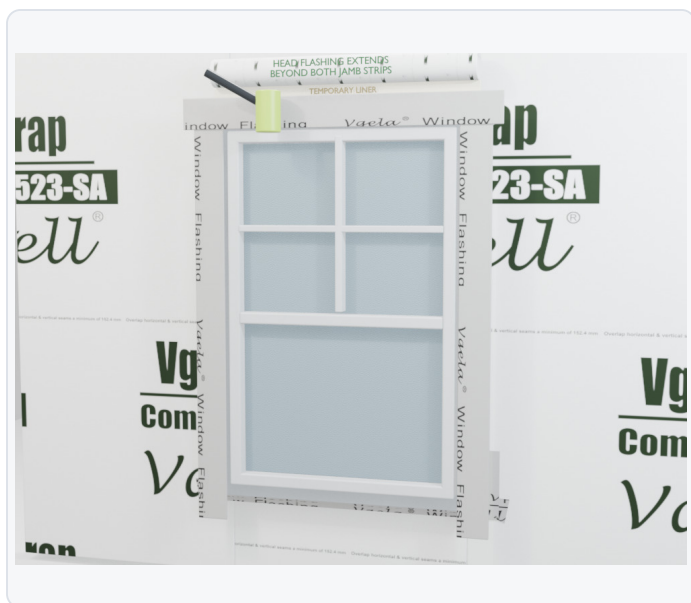
FIG 14 Head flashing overlaps beyond both jamb flashings.
