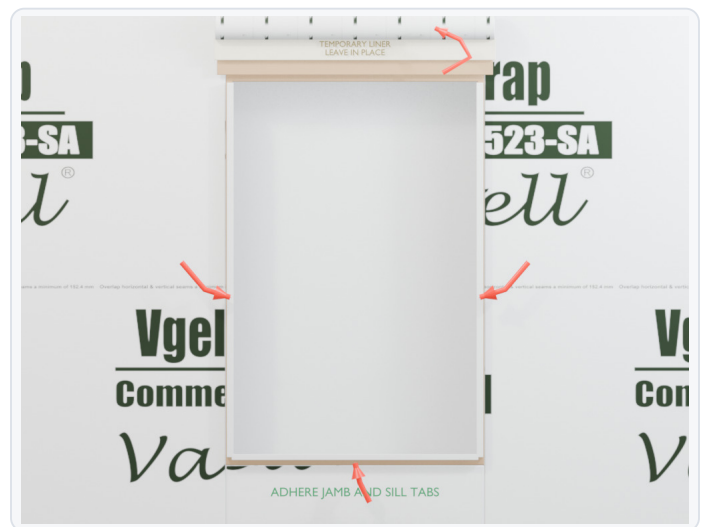
FIG 2 Fold the head flap upward; adhere jamb and sill tabs.
