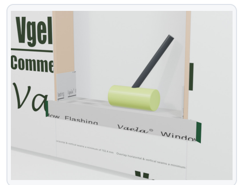
FIG 10 Cover the sill to its inside edge and roll.
