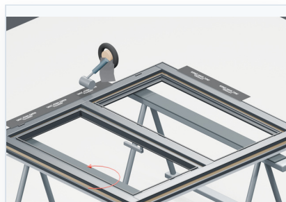
Figure 6. Exterior-side pre-application after turning the frame over.
